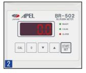
After warming-up (2min), seting "0" using a capillary tube with distilled water.
