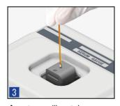
Insert a capillary tube (containing a sample) into the holder.
